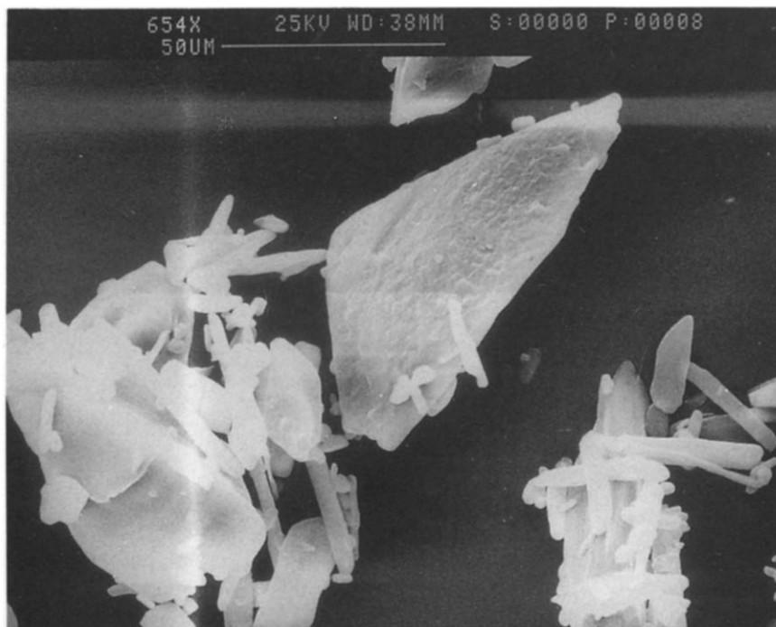
Fig. 5. Scanning electron micrograph of the surfaces of paracetamol crystals used as starting material.
